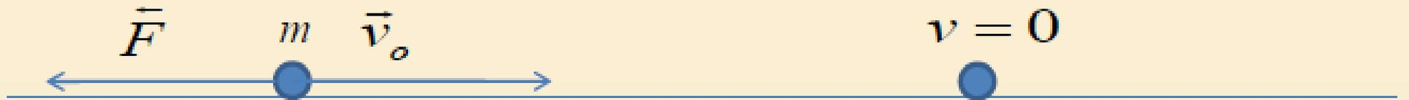
$$a = F / m \quad d_{arr} = \frac{v_0^2}{2a} \quad \leftarrow \quad L = -d_{arr} F = -\frac{v_0^2}{2a} F = -\frac{1}{2} m v_0^2$$
