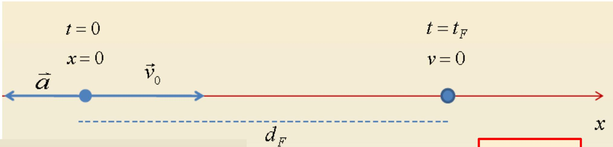
$$\begin{cases} a_x = \text{cost} = a_{0x} \\ v_x = a_{0x}t + v_{0x} \\ x = \frac{1}{2}a_{0x}t^2 + v_{0x}t + x_0 \end{cases}$$
