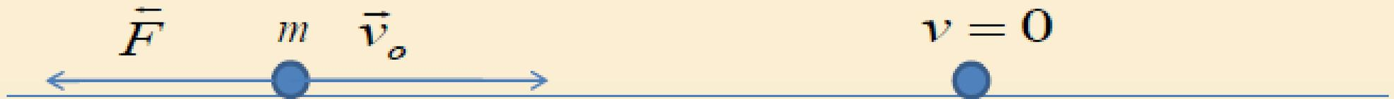
$$a = F / m \qquad d_{arr} = \frac{v_0^2}{2a} \quad \leftarrow \qquad L = -d_{arr} F = -\frac{v_0^2}{2a} F = -\frac{1}{2} m v_0^2$$
